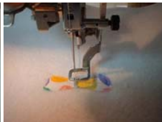
5. Place fabric over placement stitching then sew second placement. Trim around stitching. 6. Sew next colors stopping at
